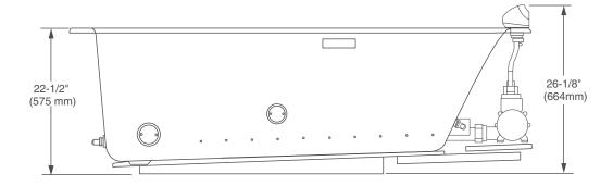
Dimensions of fixtures are nominal and may vary within the range of tolerances established by CSA B45.5/IAPMO Z124
